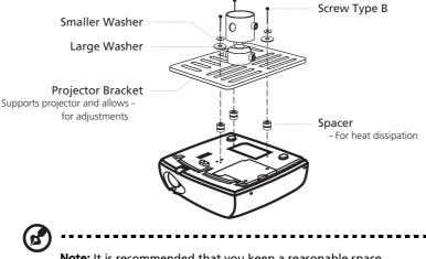
**Note:** It is recommended that you keep a reasonable space between the bracket and the projector to allow for proper heat distribution. Use two washers for extra support, if deemed necessary.
