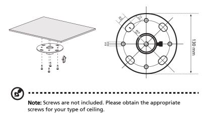
2 Secure the ceiling rod using the appropriate type of four-cylinder screws.
